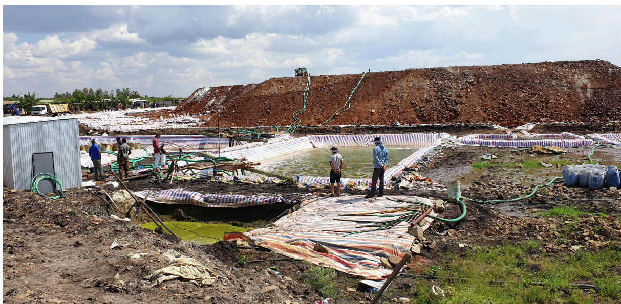
A gold leaching site in Migori county, Kenya, that uses sodium cyanide to extract gold from waste products of previous gold mining. Sodium cyanide can contaminate water sources if the proper precautions to secure leaching sites are not followed.
