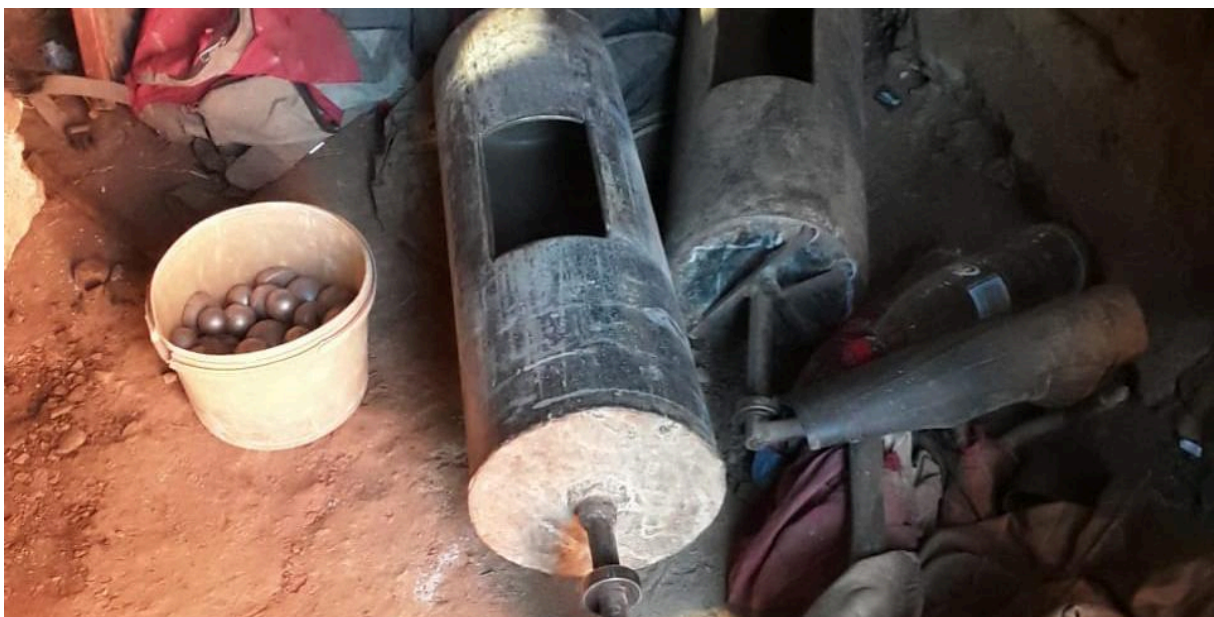
Simple equipment for processing gold ore. The cylindrical pieces of equipment are known as phendukas, which along with the ball bearings (pictured in the bucket), are used to break up the rock before processing and extracting the gold.
